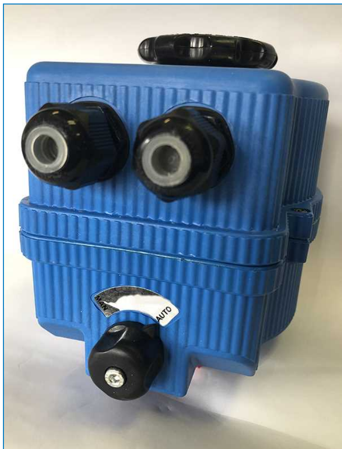
Purge valve actuator position "AUTO"
