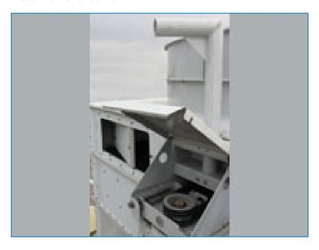
With the motor removal davit, lowering or lifting your motor from/onto the unit top is easy!
