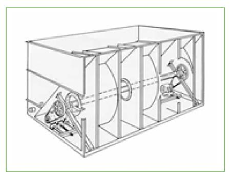
The installation of a Baltiguard<sup>®</sup> drive system
